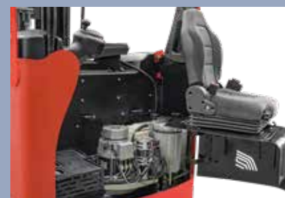
Fully open door enables easy repair and maintenance
