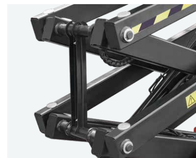
Supporting arms, To protect the operator when he is doing repair or maintenance job
