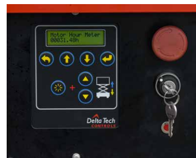
LCD screen, used to display fault code and adjust parameters
